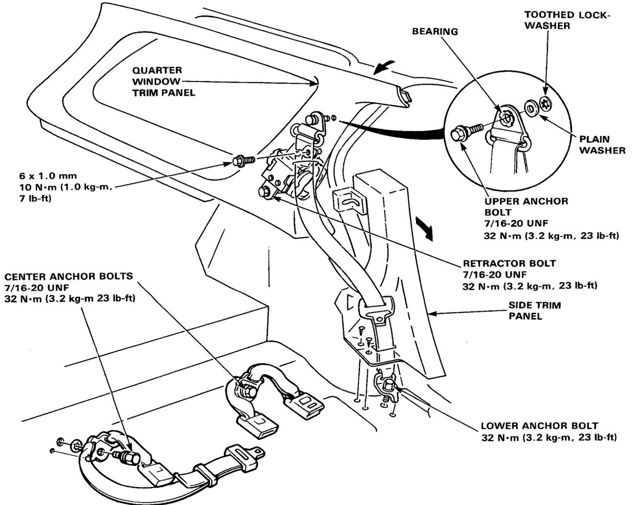
3. Check that the retractor locking mechanism functions properly.
