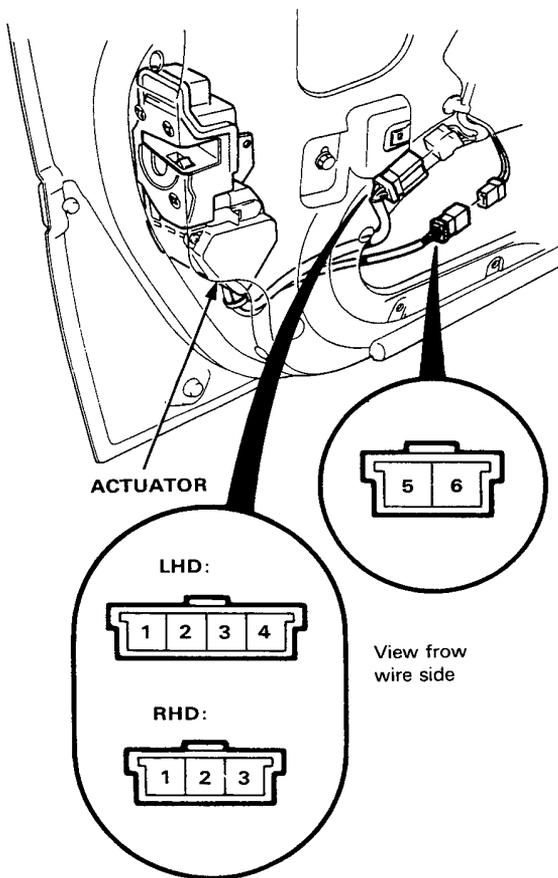
4. If the actuator fails to operate properly, replace it.
