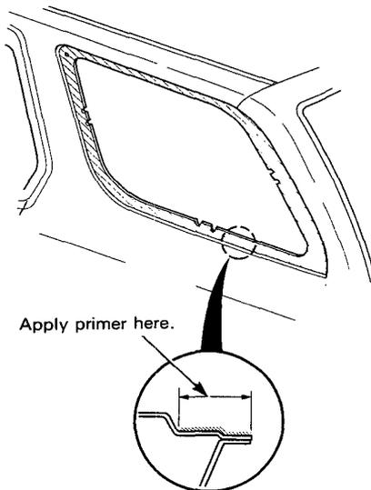
6. With a sponge, apply a light coat of glass primer around the edge of the glass as shown, then lightly wipe it off with gauze or cheesecloth.
