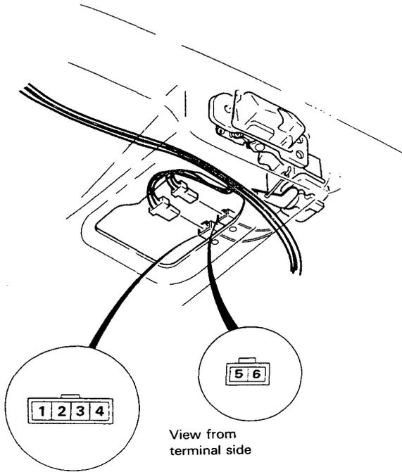
5. Check for continuity between the terminals in each switch position according to the table.
