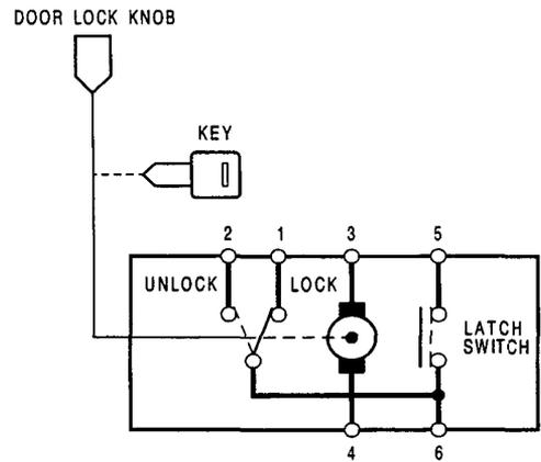
4. If the actuator fails to operate properly, replace it.
