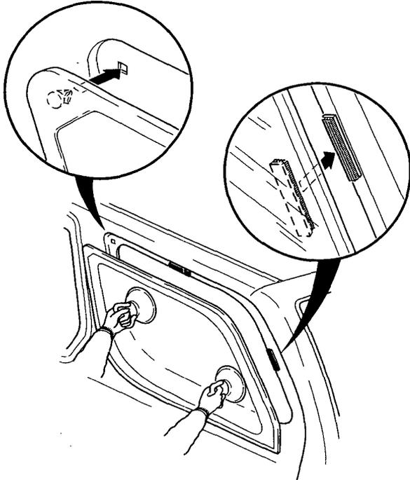
12. Scrape or wipe the excess adhesive off with a putty knife or gauze.
