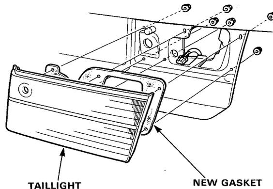
4. Inspect the gasket; replace if it is distorted or overly compressed.
