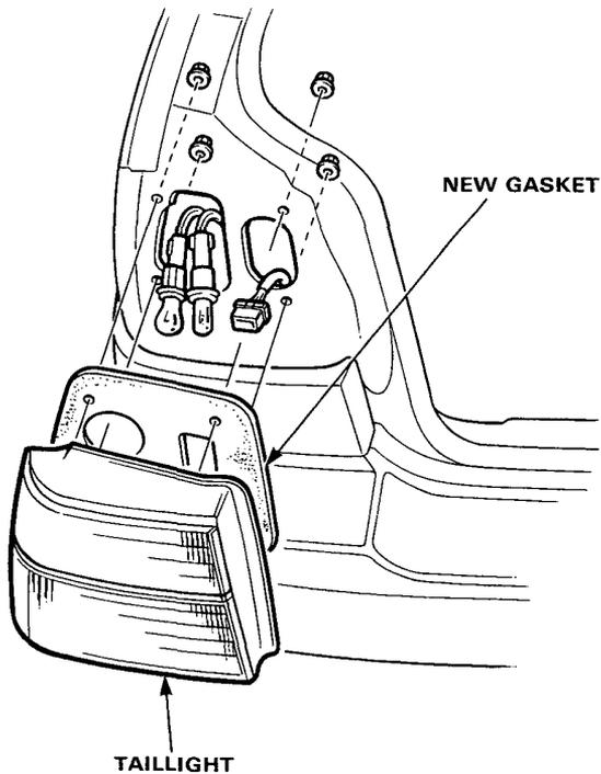
4. Inspect the gasket; replace if it is distorted or overly compressed.
