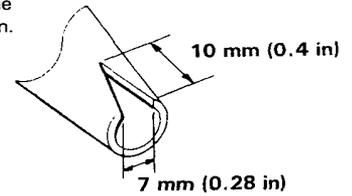
10. Pack adhesive into the cartridge without air pockets, to ensure continuous delivery. Put the cartridge in a caulking gun, and run a bead of adhesive around the edge of the glass as shown.
