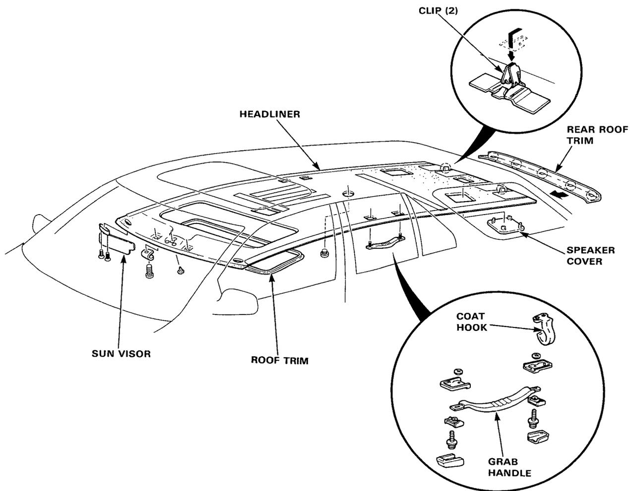
3. Assemble the headliner in the reverse order of disassembly.
